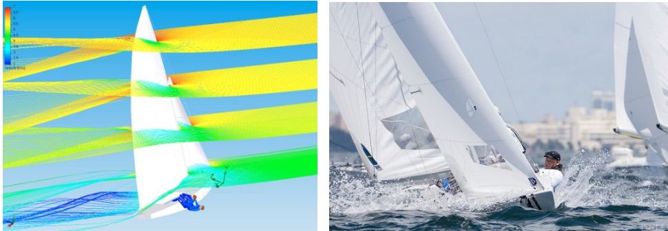
Figure 7: Medal Winning Summer Olympic Finn Class Sailing Simulation in FloEFD for the Swedish Olympic Team (Courtesy of WB Sails)
